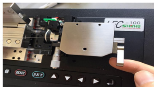
Clamp the fiber and take up handle
