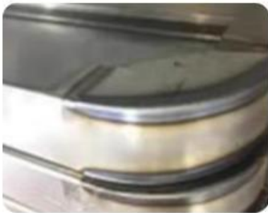
SHEET METAL OUTER CORNER WELDING
