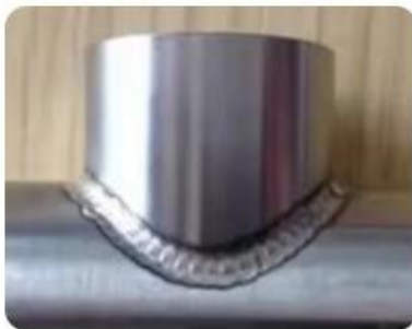
INSIDE CORNER WELDING
