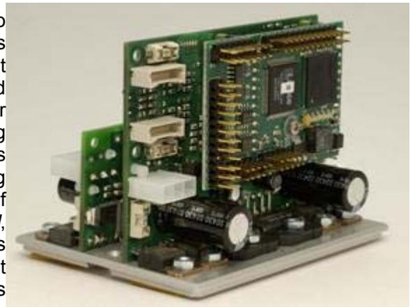
The DC servos can be used with the 6200H family of galvos. The DC900 will work with all the 6200 family and the DC2000 will work with all except for the 6200 & 6210. Also, the DC2000 will only accept XY2-100 or DAC input while the DC900 will accept Analog, XY2-100 and DAC.
